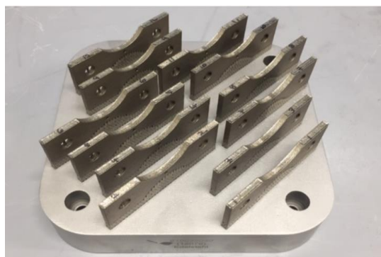
Figure 13. Fatigue test samples printed as a part of a Master thesis [2]
