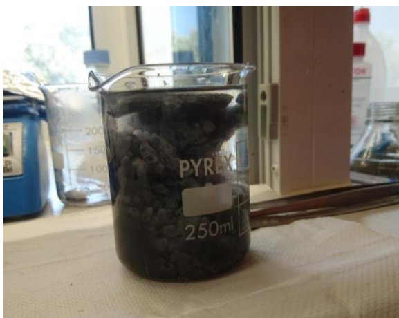
Figure 1. Solvent – based method; Dissolved LDPE inside toluene solvent with GnP filler
