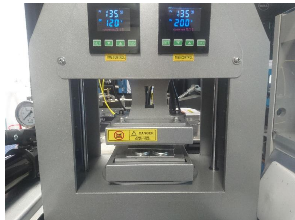
Figure 2. Hot pressing of the produced nanocomposite via solvent method into molds
