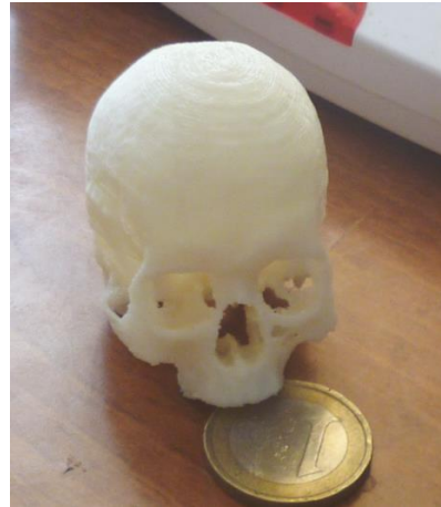
Figure 7. 1:5 scale model of the Saint skull, build to evaluate the model and the process accuracy and feasibility.
