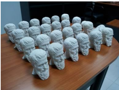
(d) Clay copies of the bust produced with the silicon rubber mould.
