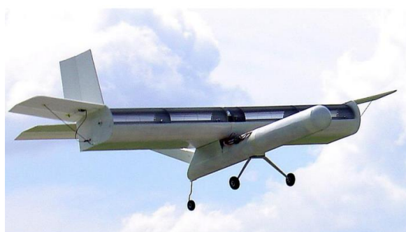
Figure 4. "FanWing" drone with electric propulsion [19]
